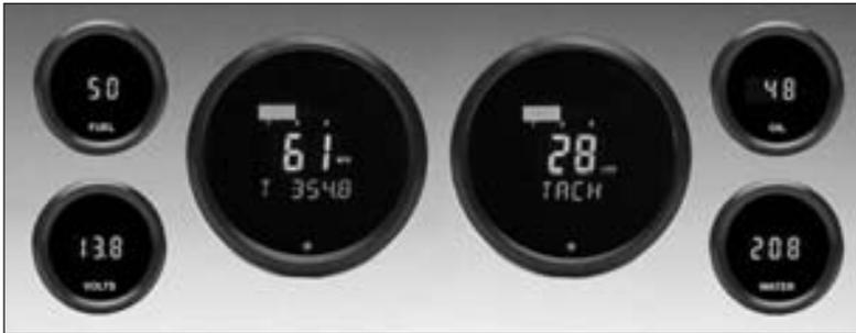
**Odyssey Series II** is the first to provide a vacuum fluorescent digital readout industry standard 3-3/8" and 2-1/16" diameter housings. Using a high contrast, non-glare, scratch resistant lens, excellent daytime visibility is achieved. The instruments automatically dim down for night driving and have a completely backlit annunciator for a black out effect when off. Odyssey Series II is backed by a 24 month warranty.
